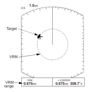
Figure 2-8 Measuring range by the VRM
